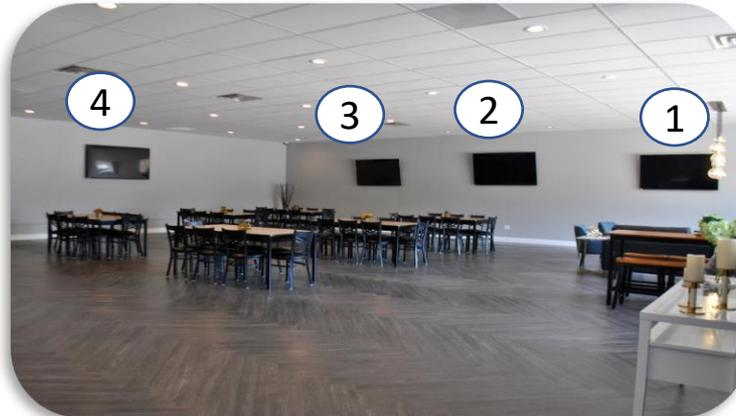
**Example 2** – To play Laptop for Slideshows or PowerPoint on all four TVs, connect HDMI Cable to Laptop. Press “HDMI” > Output #1 (i.e., TV 1) > then Input 1 (Laptop). Repeat these steps for Output #2, Output #3, and Output #4.
