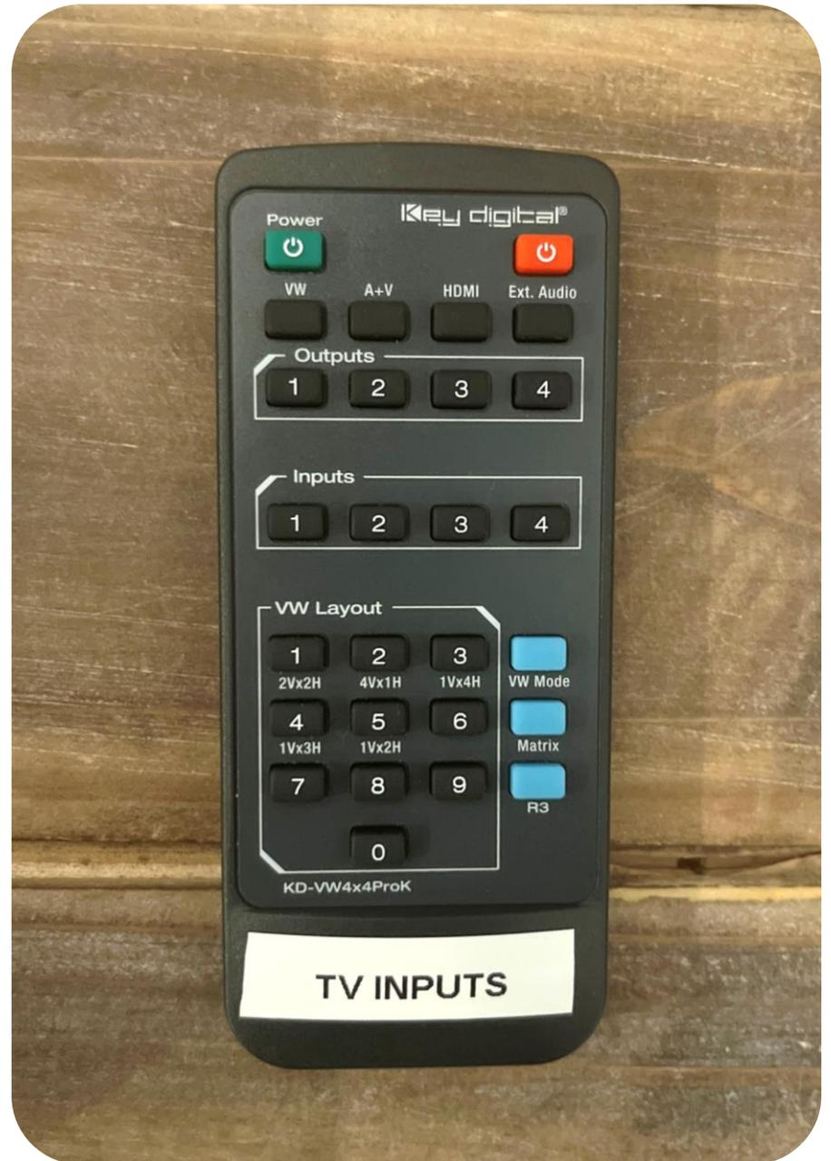
There are **three sources (INPUTS)** that connect to each TV (**i.e., OUTPUTS**) to display content – you can display these on all four TVs or on select TVs
